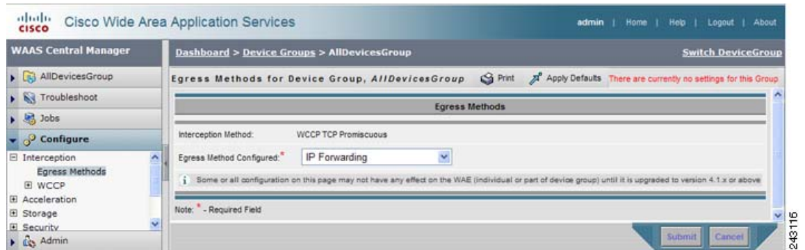
Figure 3-1 Example of a Window that Has Not Been Configured for a Device Group
